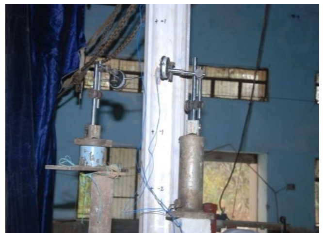
Fig 2.3. Connection of Dial Test Indicators Laterally
