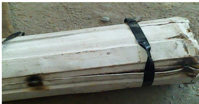
4(d) Failure of column CFSFC L/D 20 at bottom with 3/#8
