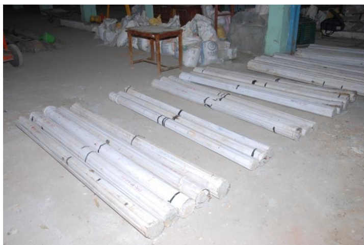
4(a). Failure of all columns ( buckling does not exist)
