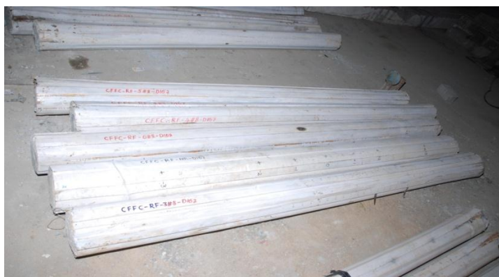
4 (b). Failure of columns at edges for L/D 15
